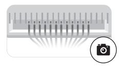
Exposed sprinkler wires with 24VAC could generate an electric shock in wet locations. Please ask your retailer or contractor if sprinkler accessories may be needed.
